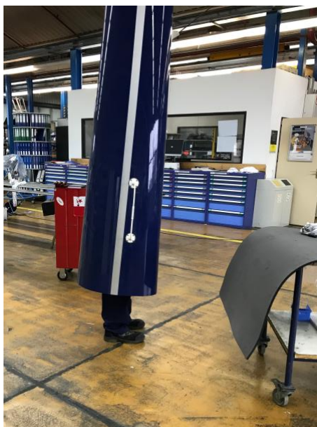
Innen-Kontrolle Tailboom EC120
